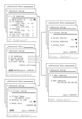
**DHCP** (**Dynamic Host Configuration Protocol**) and **AutoIP** are mechanisms for network configuration, which assign IP addresses automatically to the network devices such as the DTR-8.3, PC, and broadband router.
